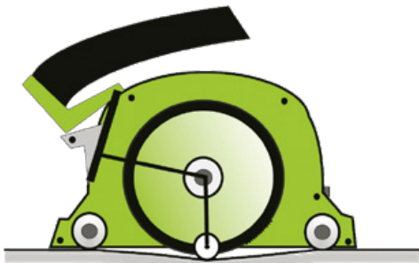
Principle of automatic depth control
